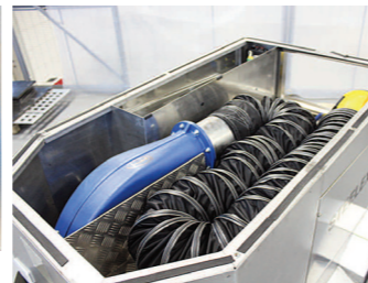
Heater hose is stored inside the heater chassis.
