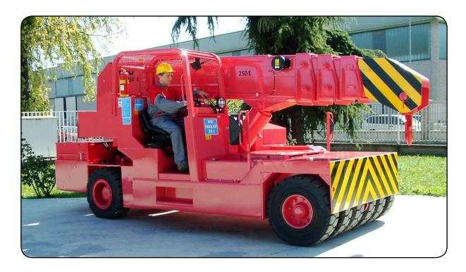
**PROPULSION:** 28 kW - 96 V DC fanned reversible electric motor fitted with a MOSFET speed control and microprocessor. Foot operated brakes on 6 wheels. Hand brake hydraulically operated.
