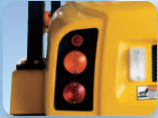
Backup light and buzzer for safe reversing
