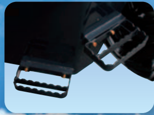
Two-stage step for safe mounting/dismounting
