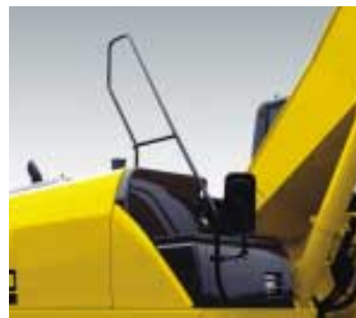
ISO-compliant large handrail
