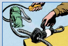
Wire rope, cable cutting
