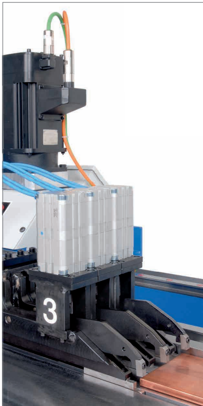
1-3 exchangeable clamps are used depending on the width of the bar
