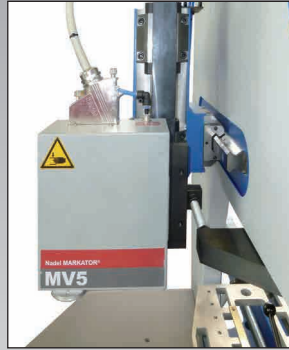
CU Profi and CU WK II marking unit: for labeling of finished parts
