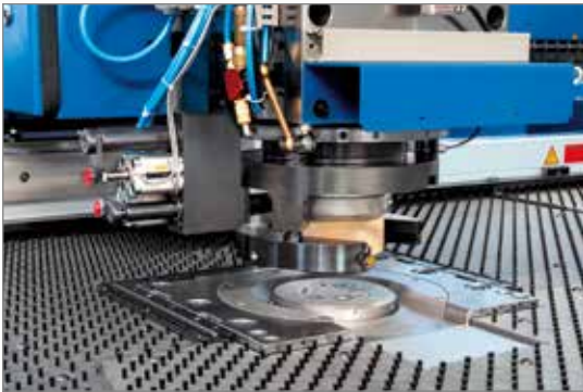
Punching head rotation Index equipment and also stripper height adjustment
