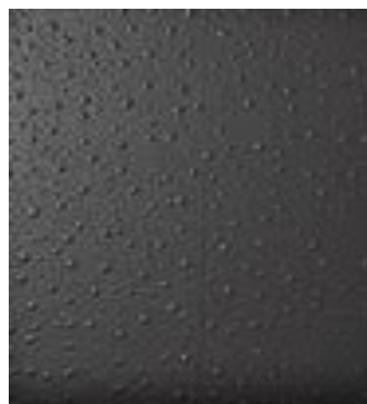
Commercial Benchmark 2 coats - 750 hours salt fog cold rolled steel
