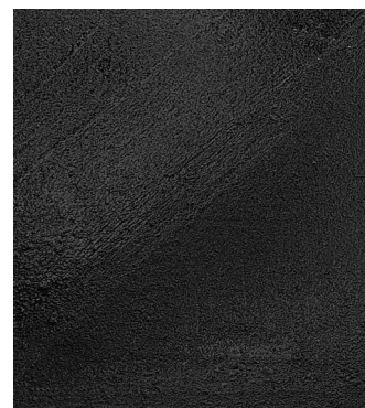
Neutrurust 661® Technology 2 coats - 750 hours salt fog cold rolled steel
