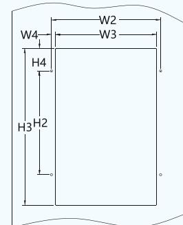
380V 90-110kW VFD flange installation diagram
