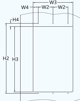
380V 132-200kW VFD flange installation diagram
