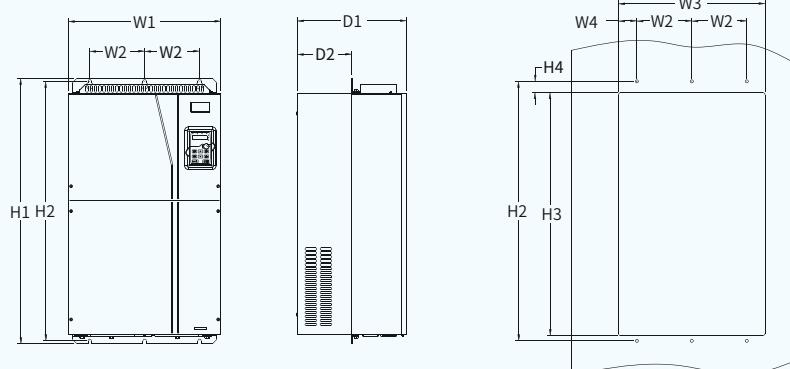
660V 160–220kW VFD flange installation diagram
