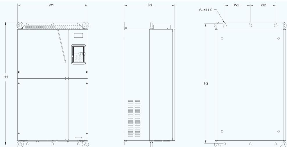
380V 132-200kW VFD wall mounting diagram
