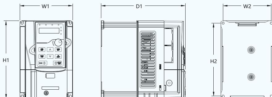
380V 1.5-37kW VFD wall mounting diagram
