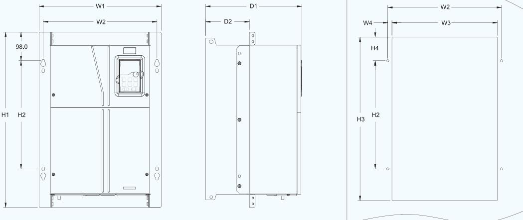
660V 22–132kW VFD flange installation diagram
