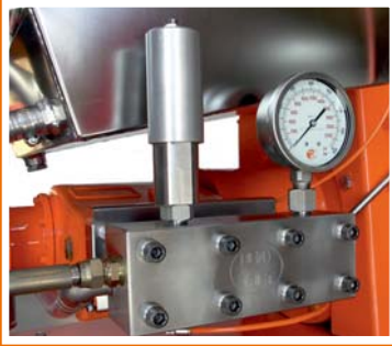
Stainless steel pump-head. Integrated cooling for plunger-seals.
