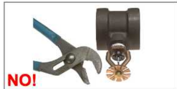
Figure 2: Incorrect installation wrench (ESFR sprinkler shown with Channel Locks)
