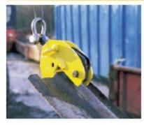
The PP pile pulling clamps are designed to pull out driven piles or trench shielding. The clamps have a narrow opening and a deep slot to ensure that the pile is gripped firmly. It is extremely difficult to determine the forces required to pull out driven piles so it is recommended that a load indicator is used to ensure the WLL of the clamp is not exceeded.
