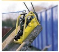
The CP pile pitching clamps are specifically designed for pitching sheet steel piling. These clamps come fitted with a 15 metre length of rope which allows the clamp to be release from the ground. These units also come fitted as standard with a shackle.
