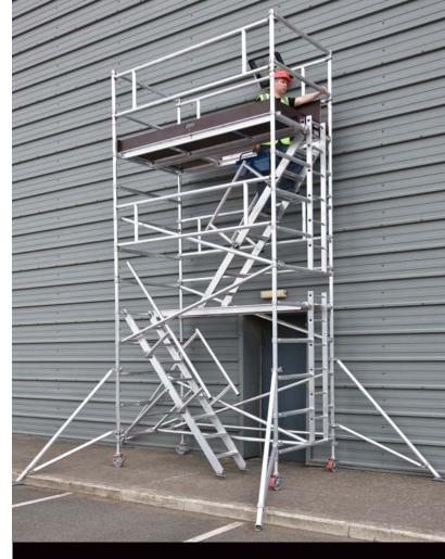
The Instant Stairway tower is a versatile unit which can easily convert both a standard Span 300 and a Span 400 mobile access tower into a stairway tower. It provides safe landings every 2 metres. Stairway steps are 145mm deep, with a clear width of 450mm making it easy to carry tools. The step rise is 230mm and the angle of inclination is 51 degrees.
